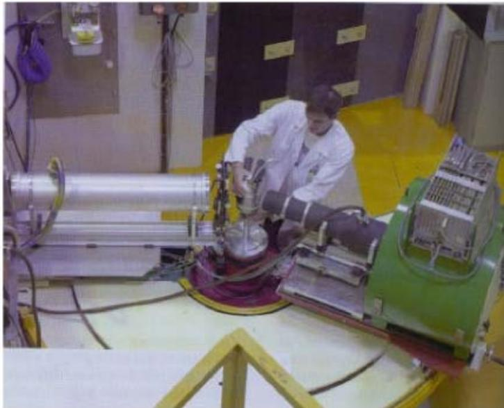
Note: relatively massive shielding; long flight paths for time-of-flight spectrometers; many or multi-detectors on modern instruments
