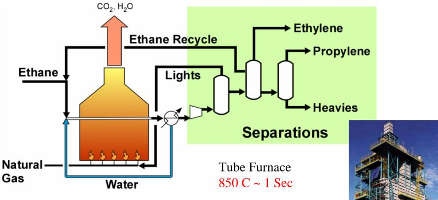
$C_{2}H_{6} + O_{2}$  (Air) Feed:  $C_2H_4 + C_3H_6 + Heavies + H_2O + CO_2$ Products:
